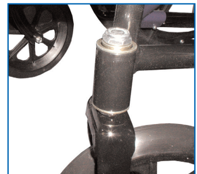
Precision seal bearing in all key locations provides smooth noise free operation.
