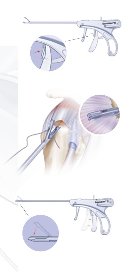
**3.** Open the jaw by pushing the jaw release button.
