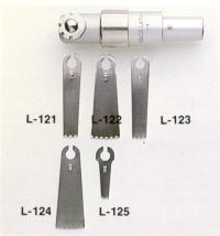
The saw insert can be engaged into the handpiece in four positions. Blades can be attached in five positions No tools are required to attach or remove blades. Blades oscillate at 11,000\*cycles per minute with a maximum 1/4 inch excursion arc.
