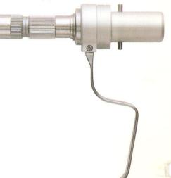
The quick-release chuck lever allows pin insertion and advancement without the use of additional keys and accessories. Internal cannulation of insert will accommodate wires and pins from 1/16 inch (1.6 mm) to 5/32 inch (4.0 mm).
