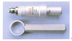
• Fully cannulated, insert develops low speed and high torque for heavy duty reaming; reduces Maxi-Driver II system speed to 250 rpm. Stall torque: 115 in-lb
