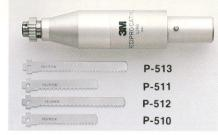
The saw insert can be engaged into the handpiece in four positions. Blades can be inserted in two positions. No tools are needed to insert or remove the blades. Positive blade locking mechanism minimizes chance of blades disengaging during surgery. Blades reciprocate at 3000 strokes per minute with a 1/4 inch stroke.
