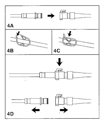
Figure 4—Colder-style Connectors
