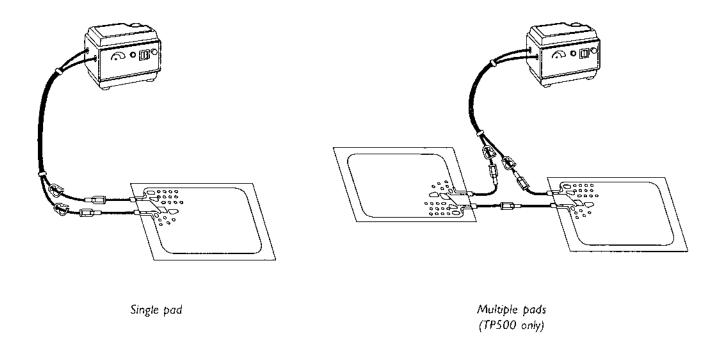
Figure 1—T/Pump Heat Therapy System
