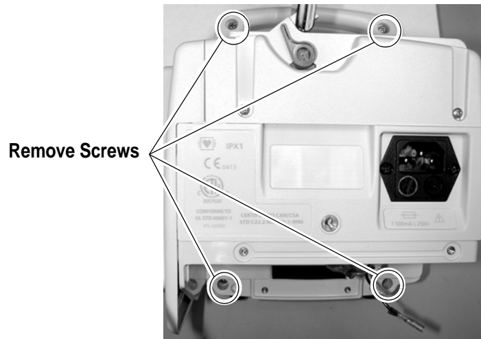
Figure 7-49: Remove Screws Holding Bezel
