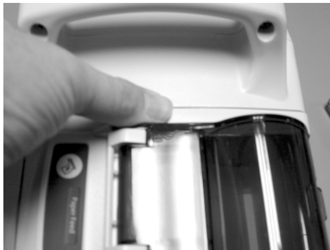
Figure 7-2: Release Printer Tab
