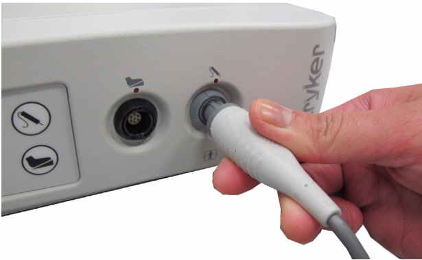
Figure 4: Connecting the Probe to the Generator
