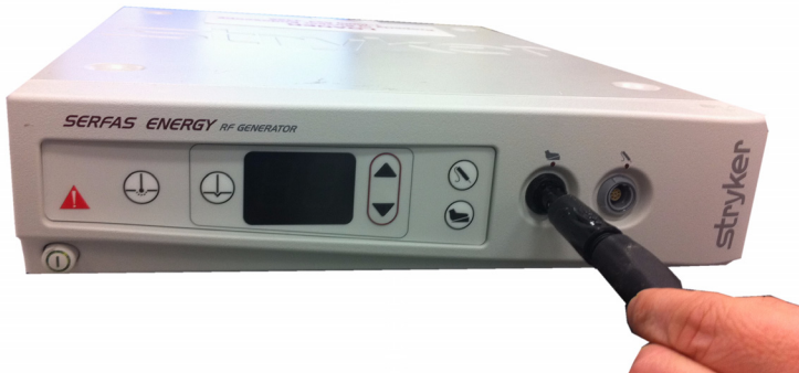
Figure 5: Connecting the Footswitch to the Generator
