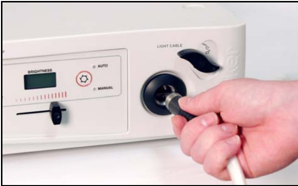
Figure 4: Inserting the light cable into the cable port
