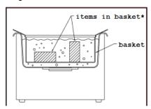
\*The item(s) to be cleaned are put directly into an Accessory Basket and placed into the tank
