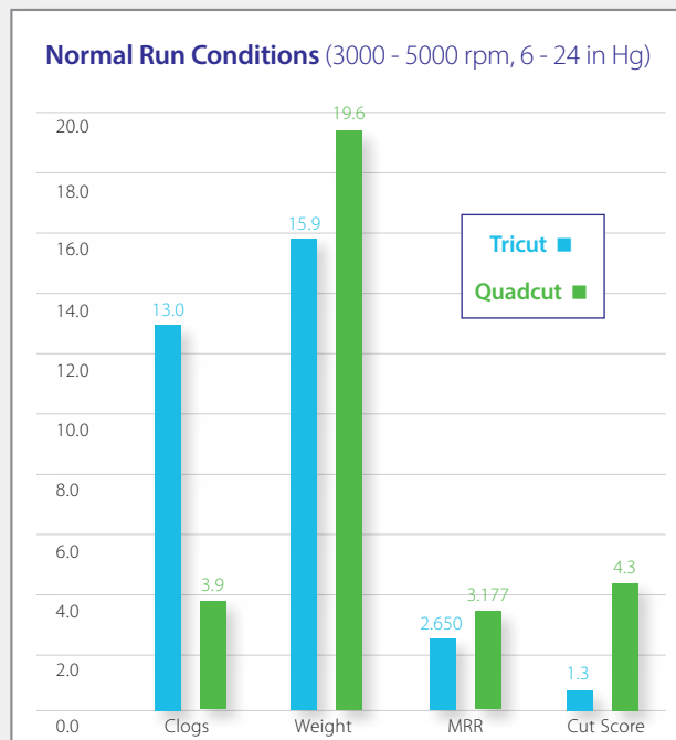
Data collected from 4.3 mm Quadcut Blade
